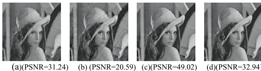
Fig. 2. Comparison of Reconstructed image (a) (b) JPEG with EEP, (c) (d) adaptive segmentation with UEP;(a)(c) E_b/N_0=1.6\text{dB} , (b)(d) E_b/N_0=1.1\text{dB}
