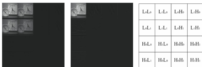
Fig. 2. Single-level decomposition of Clock image
